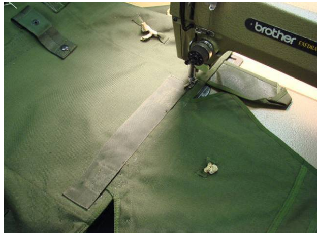
Figure 32. Re-Stitch Reinforcement Panel.
