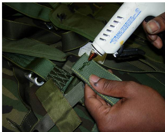
Figure 23. Apply Glue to the Upper Main Lift Web.
