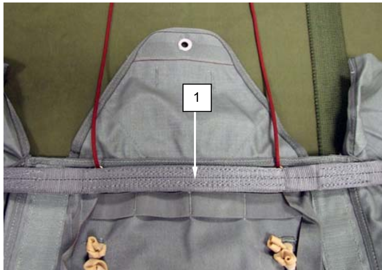
Figure 62. Centering the Spreader Bar Between Upper and Lower Grommets.
