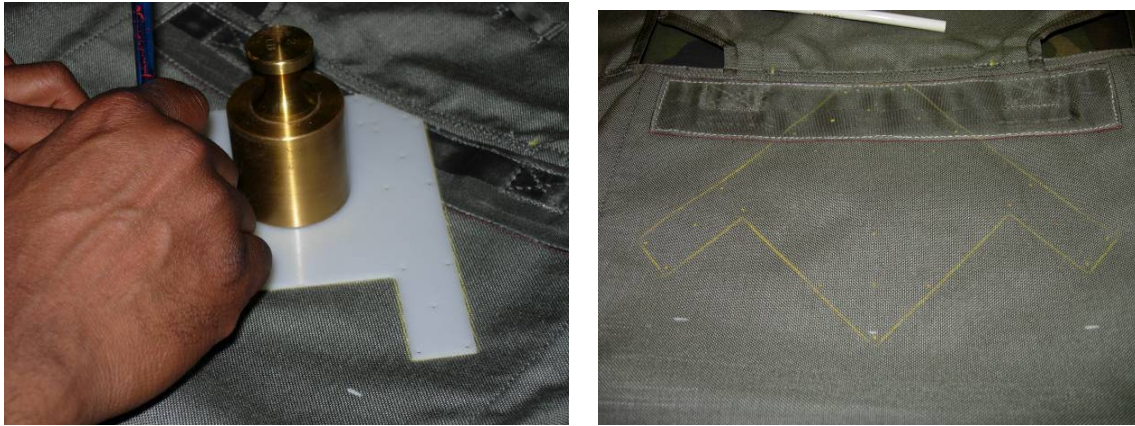
Figure 36. Trace the Outer Edge of the Template and Mark Holes.
