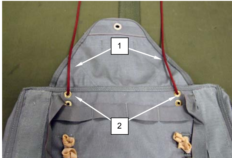
Figure 61. Route Type III Nylon Cord (RED) Through Top Grommets of Pack Tray.
