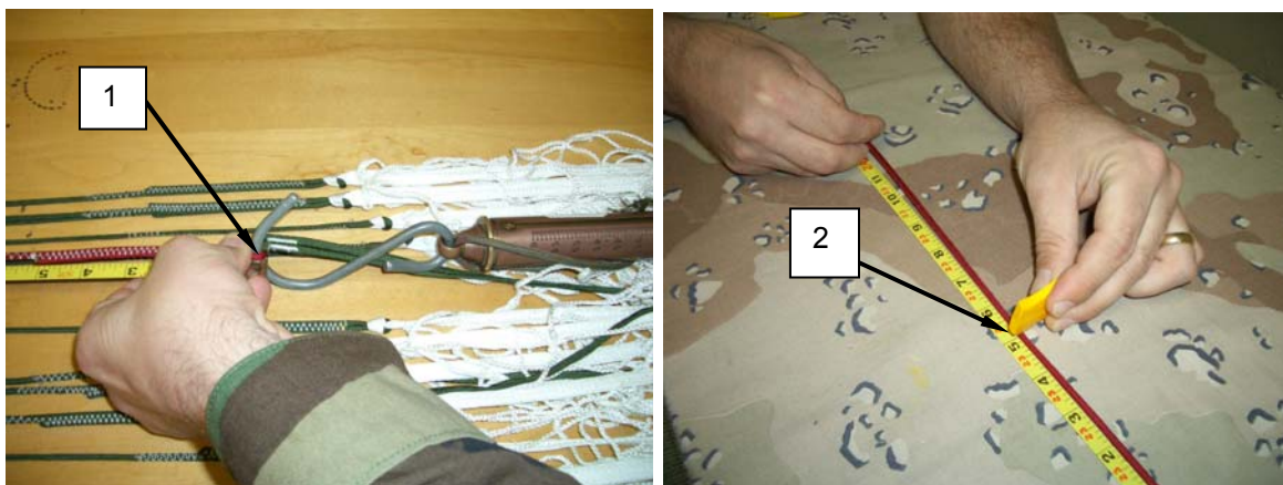
Figure 2. Marking Control Line at 282 Inches.
